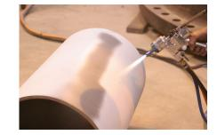
In the Arcspray process, two electrically charged wires are driven and guided so that they converge at a point and form an arc. An air nozzle atomises the molten metal produced and projects it towards the work piece. The
